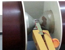
Magnetostriction and Magnetoresistance probe between poles of electromagnet
