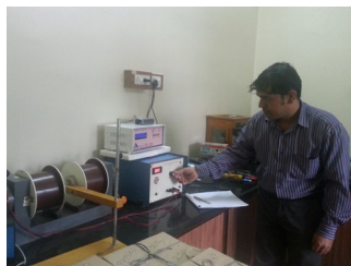
Magnetostriction and Magnetoresistance probe between poles of electromagnet
