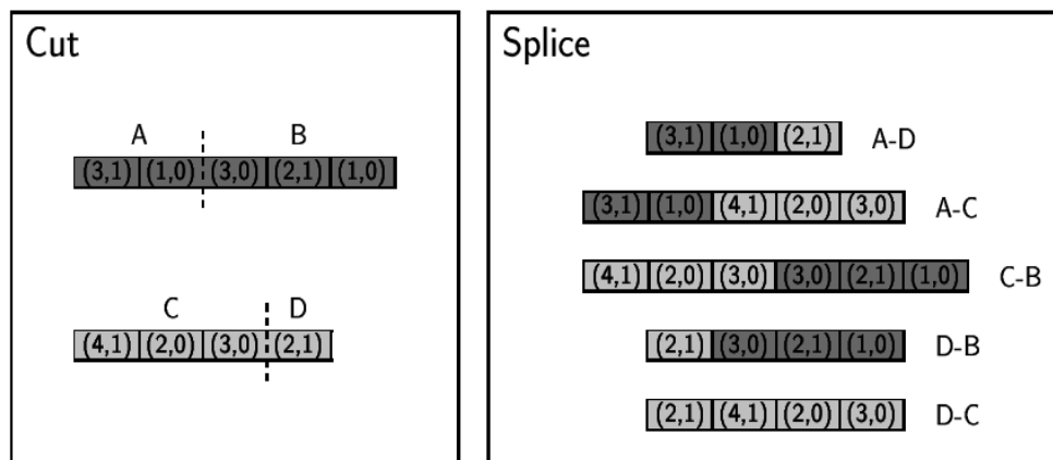
Figure 4b.21 the cut and splice operation.
