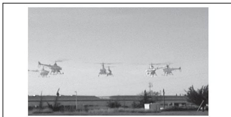
Figure 6.10 Superimposed time-lapse images of an autonomous helicopter performing a very difficult “nose-in circle” maneuver. The helicopter is
