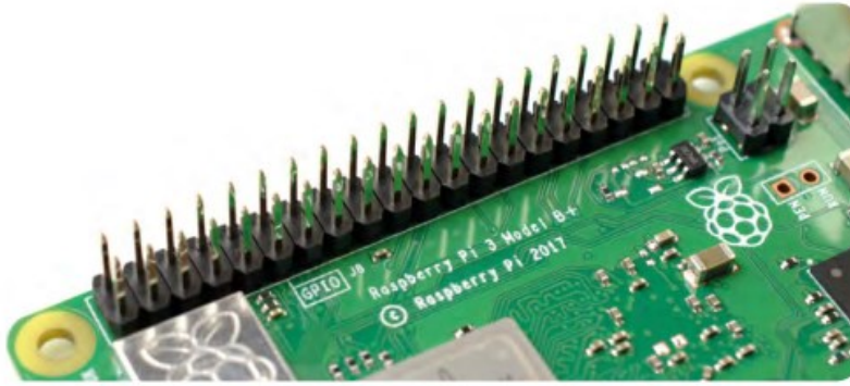
Figure 1.37 The Raspberry Pi's GPIO header
