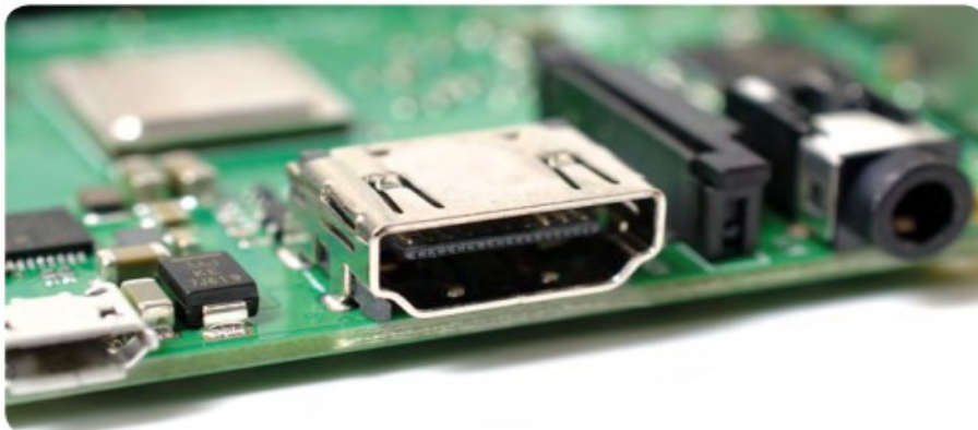
Figure 1.34 Raspberry Pi's HDMI port
