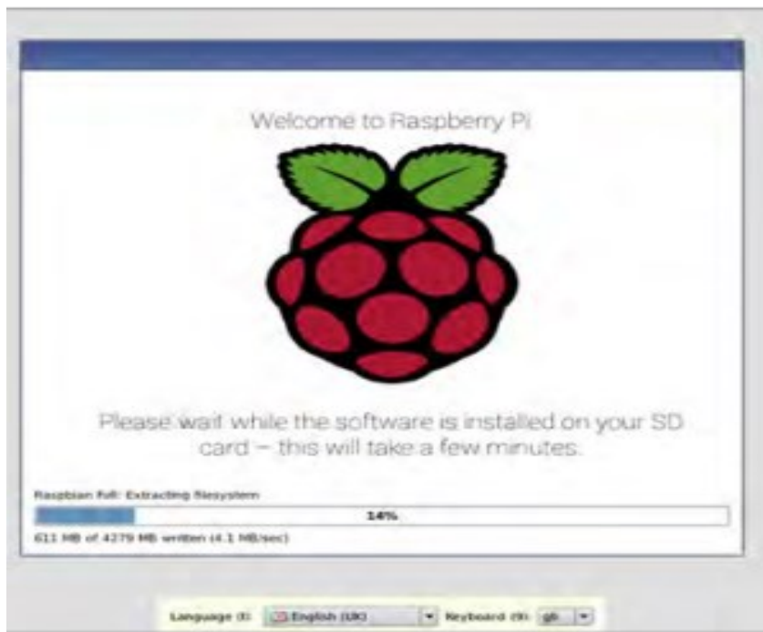
Figure 1.42 Installing the Raspbian operating system
