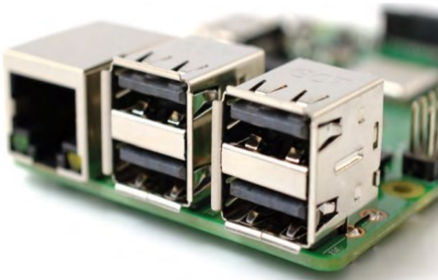
Figure 1.30 The Raspberry Pi's USB ports
