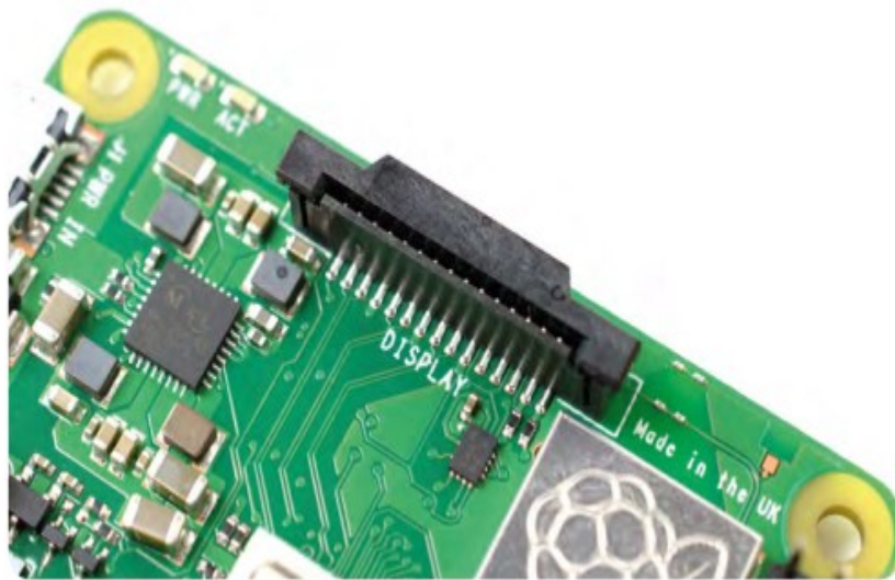
Figure 1.35 The Raspberry Pi's display connector (DSI)
