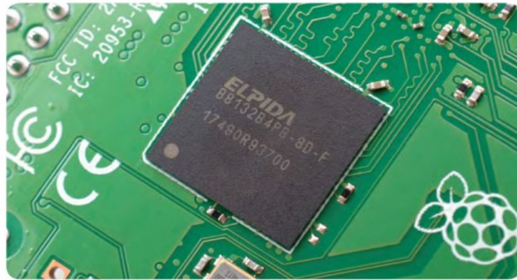
Figure 1.27 Raspberry Pi's random access memory (RAM)
