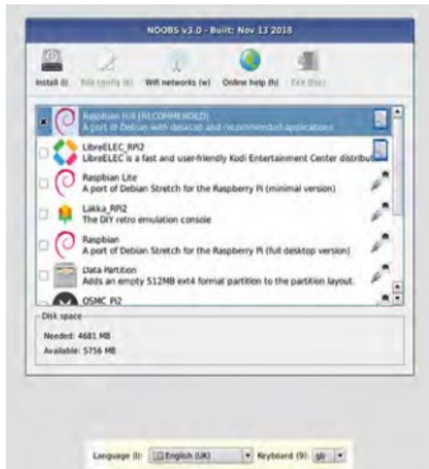
Figure 1.41 Choosing an operating system to install through NOOBS
