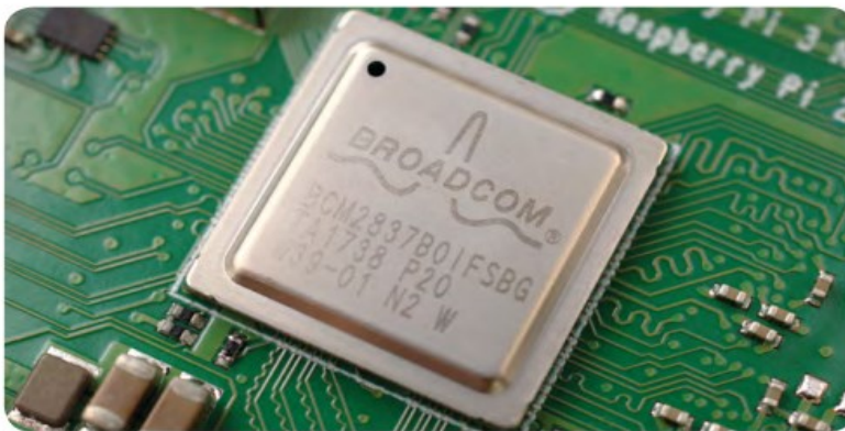
Figure 1.26 The Raspberry Pi's system-on-chip
