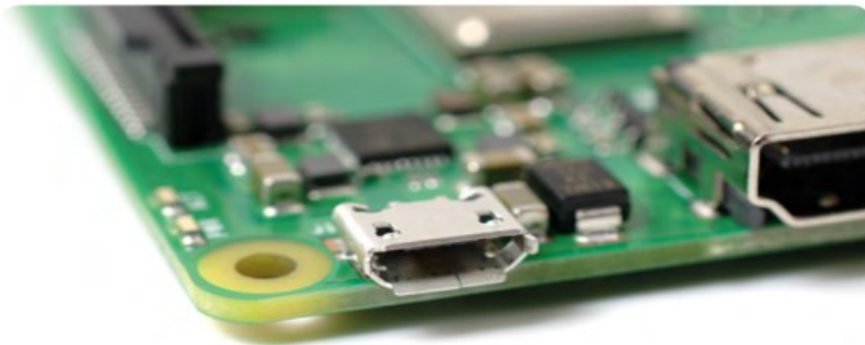
Figure 1.35 The Raspberry Pi's micro USB power port
