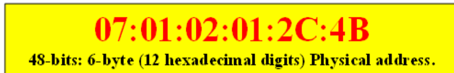
Figure 7.1: Physical address or MAC address used by Data Link layer
