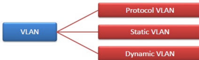
Figure 10.9: Types of VLAN
