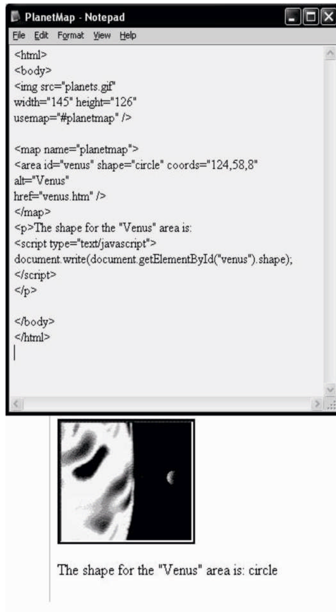
Fig 8.7 Script and output Demonstrating Area object.
