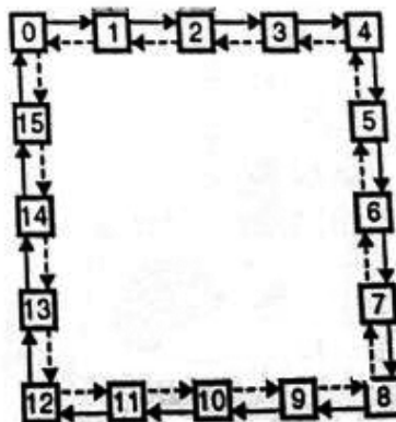
Figure 10.12.1(a): State diagram – IC 74191
